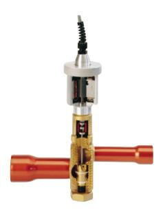
When coupled with Trane «Adaptive Control™» microprocessor, the electronic expansion valve significantly improves part load performance of the RTUA chiller by minimizing superheat in the evaporator and allowing the chiller to run at reduced condensing pressures.
